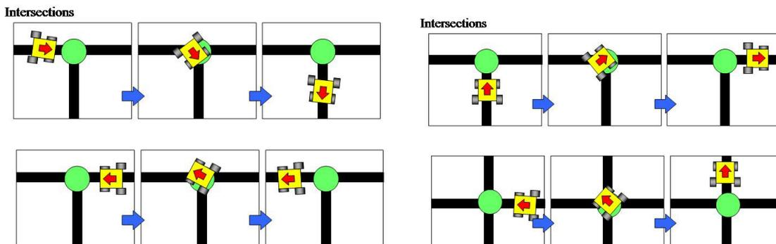
**1.6.1** Intersection Markers are green circles with an approximate radius of 2 cm, positioned over an intersection. They indicate the correct path to follow.
